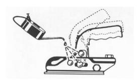
Internia brake lubrication: Lubricate with grease (see figure below) and the sliding parts with oil.
