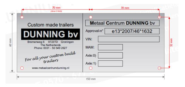
The Constructionplate is located on the drawbar on the right front leg. The VIN number is located on the upper side of the right leg and drawbar consists of 17 characters.
